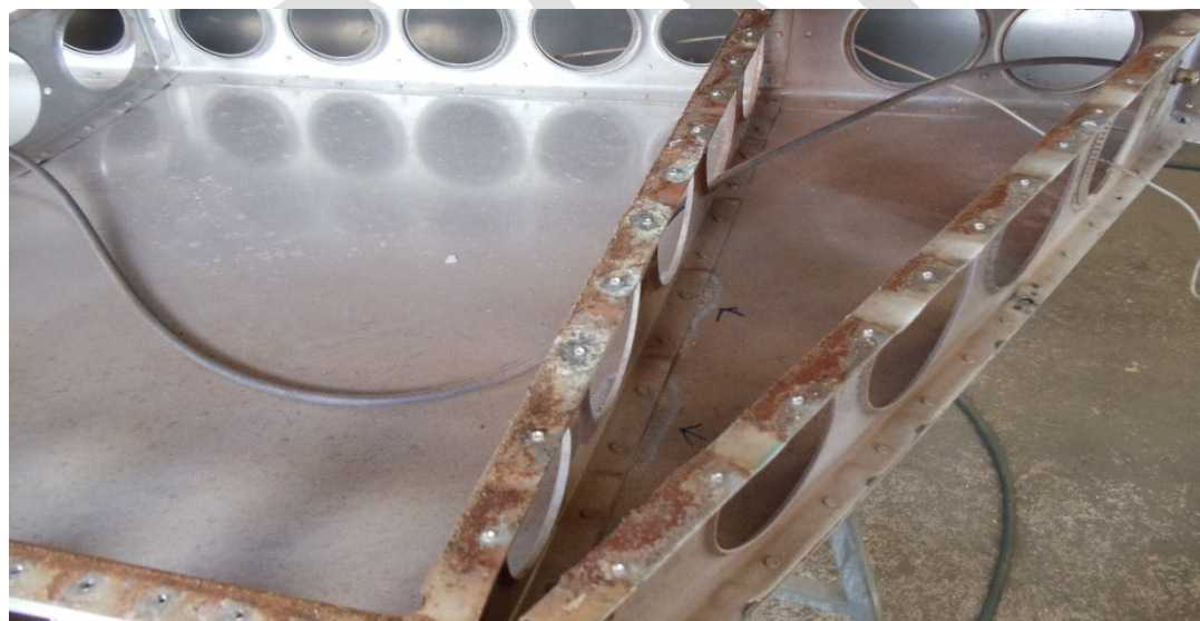
Figure 4. Cessna 152 vertical fin corrosion
