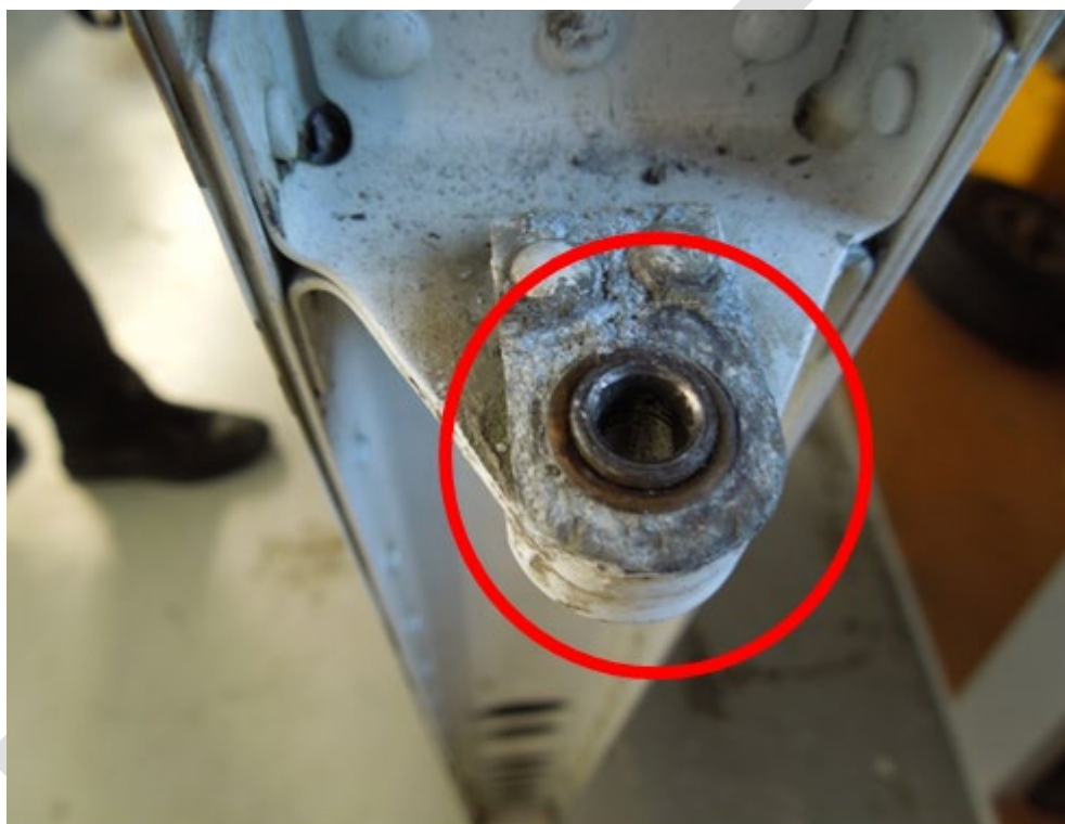
Figure 1. Centre Rudder Hinge Mount Corrosion
