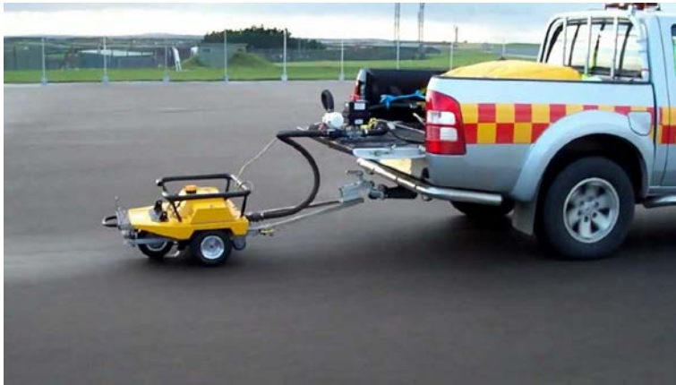
Figure 6. Example Griptester CFME in operation.
