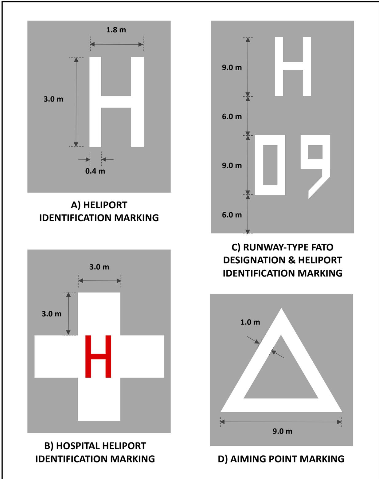
Figure 17: Heliport identification marking details
