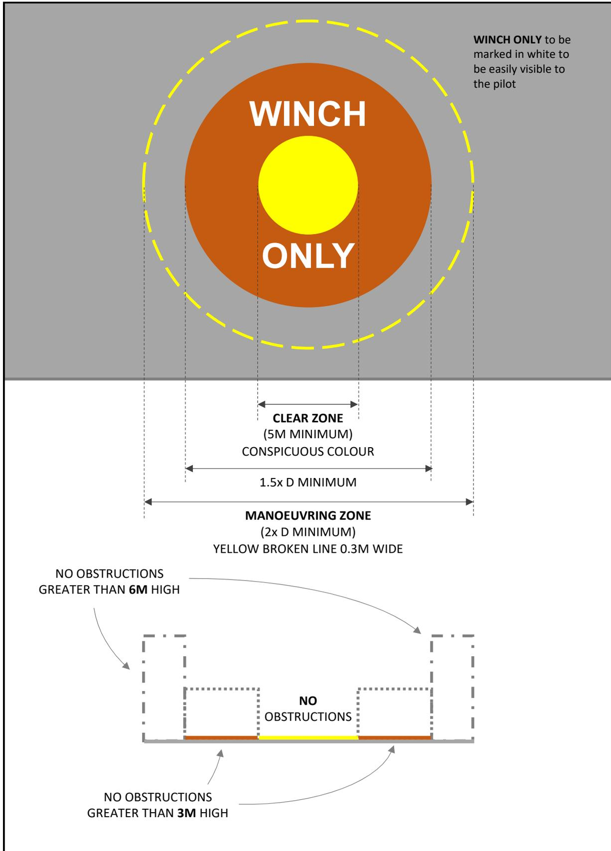
Figure 15: Shipboard winching area obstacle limitations and markings
