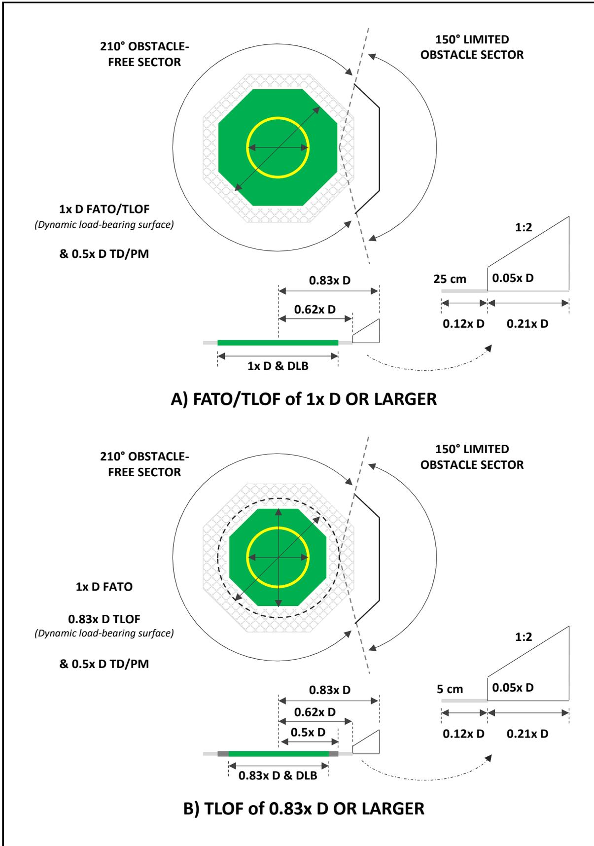
Figure 12: Helideck obstacle limitation surfaces and sectors
