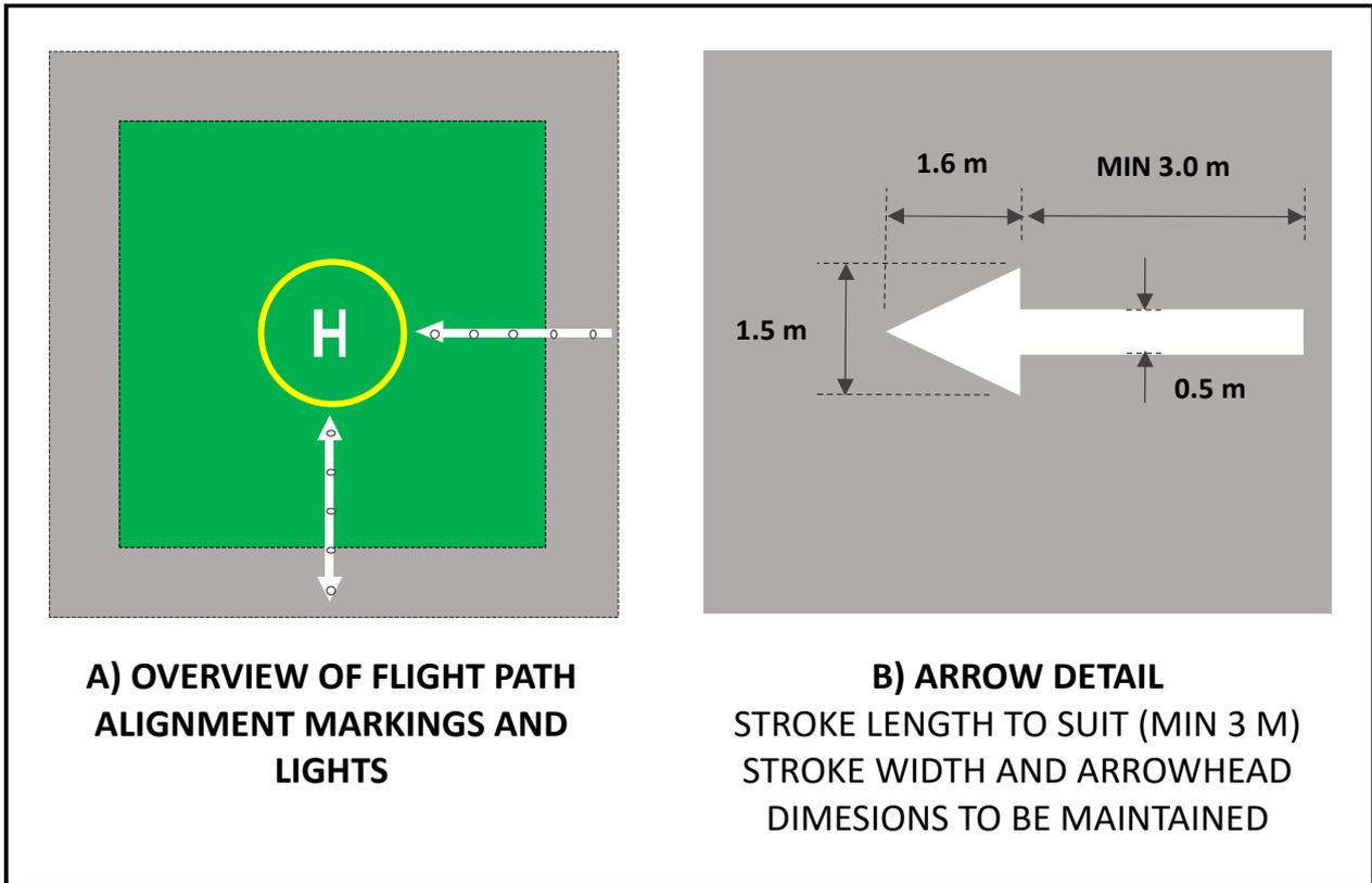
Figure 21: Flight path alignment guidance markings and lights
