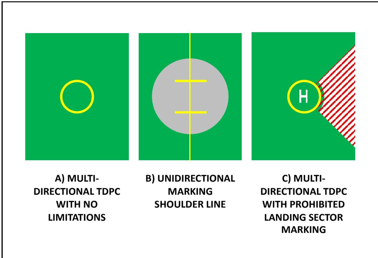
Figure 19: Examples of touchdown/positioning markings
