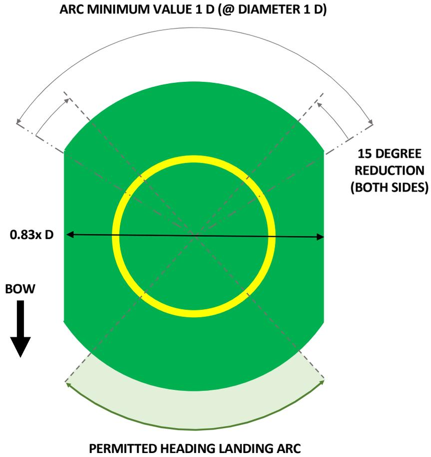
Figure 5: Shipboard permitted landing headings for limited heading operations
