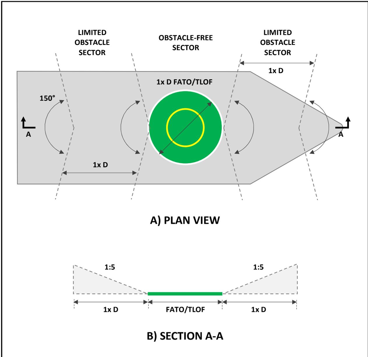
Figure 13: Amidships location – shipboard heliport obstacle limitation surfaces
